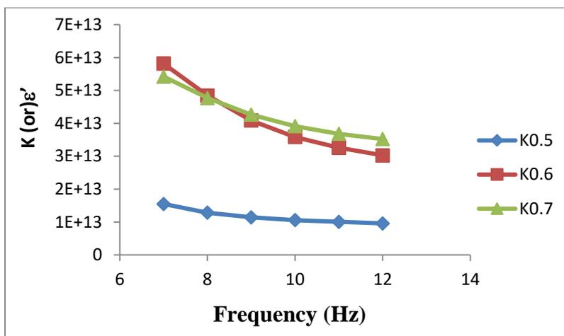
**Figure 5** Variation dielectric constant of prepared  $\text{LiNi}_{1-x}\text{Co}_x\text{O}_2$  sintered at  $900\text{ }^\circ\text{C}$  as a function of frequency at 2 V
