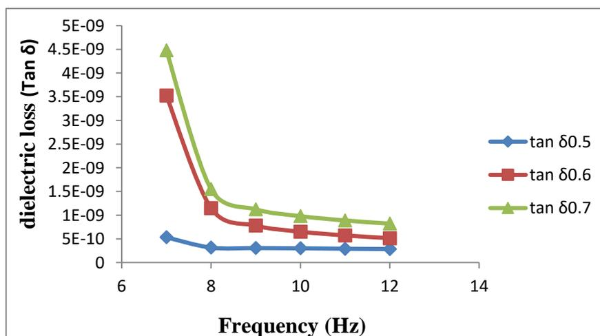
**Figure 6** Variation dielectric loss of prepared  $\text{LiNi}_{1-x}\text{Co}_x\text{O}_2$  sintered at  $900\text{ }^\circ\text{C}$  as a function of frequency at 2 V
