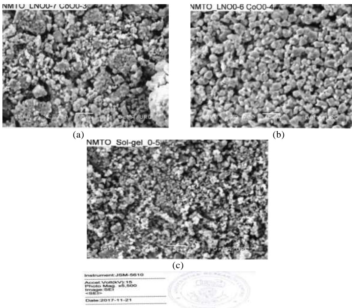
**Figure 3** SEM micrographs of (a)  $\text{LiNi}_{0.7}\text{Co}_{0.3}\text{O}_2$  (b)  $\text{LiNi}_{0.6}\text{Co}_{0.4}\text{O}_2$  and (c)  $\text{LiNi}_{0.5}\text{Co}_{0.5}\text{O}_2$  powders sintered at  $900\text{ }^\circ\text{C}$  for 4 h
