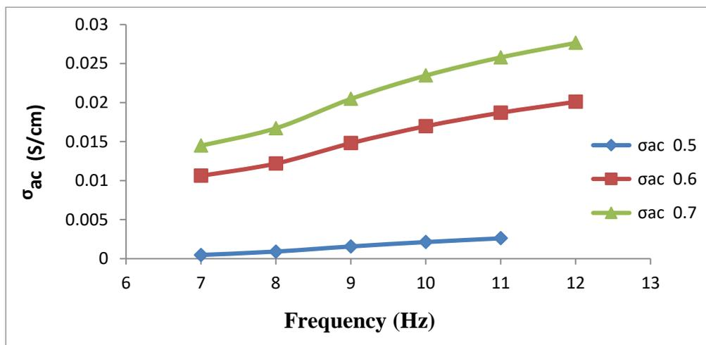
**Figure 4** Variation of ac conductivity of prepared  $\text{LiNi}_{1-x}\text{Co}_x\text{O}_2$  sintered at 900 °C as a function of frequency at 2 V**Table 4** Dielectric Constant ( $\text{Tan } \delta$ ) of Prepared  $\text{LiNi}_{1-x}\text{Co}_x\text{O}_2$  as a Function of Frequency at 2V
